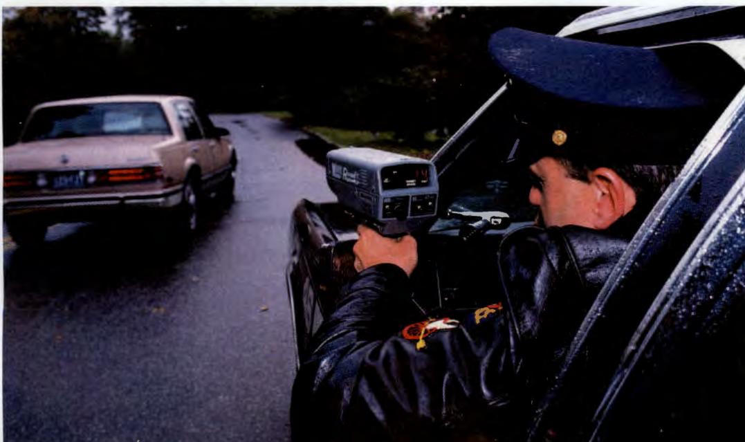
FIGURE 4 Radar Gun Radio waves are used to find the speeds of moving vehicles.
